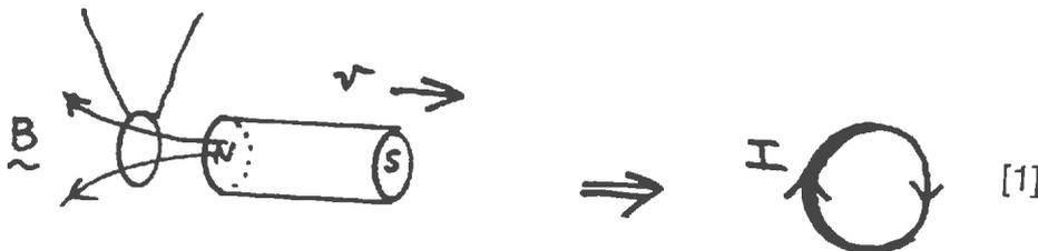
This current in the field of the magnet causes the loop to be pulled to the magnet's movement. The effective current in the North Pole of the magnet flows in the same direction - like currents attract - hence the movement. [1]
