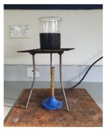
Copper oxide powder is added to **warmed** sulfuric acid until the copper oxide stops disappearing.
