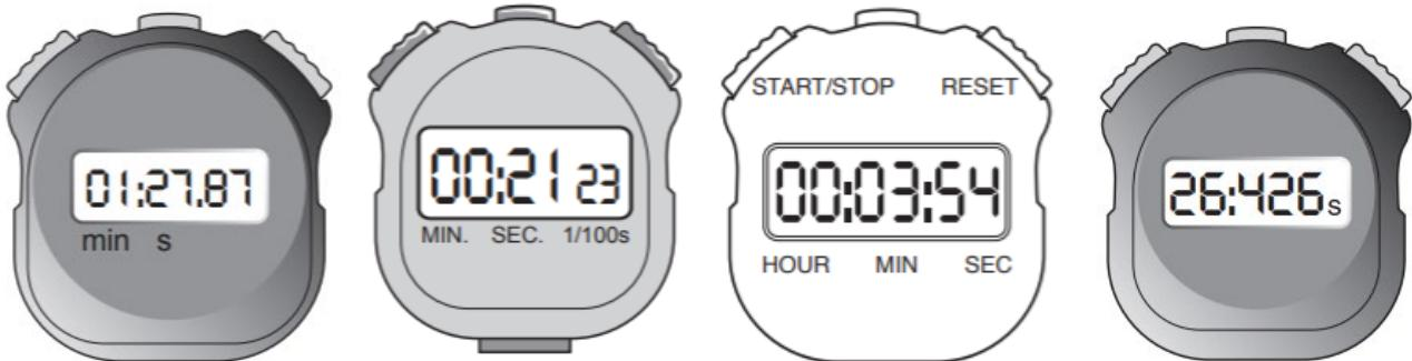
Read the stopwatches carefully e.g. min s vs hour min sec etc
