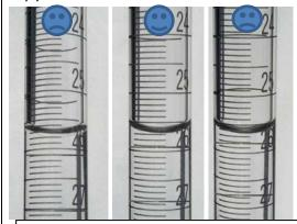
Eye is too low in the first picture and too high on the third. The middle gives correct reading of 25.65 (mL)
