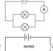
In a <u>series circuit</u> the electrical components eg bulbs are connected one after another. There is only one path for the current. When the switch
