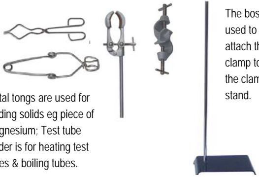
Metal tongs are used for holding solids eg piece of magnesium; Test tube holder is for heating test tubes & boiling tubes.
