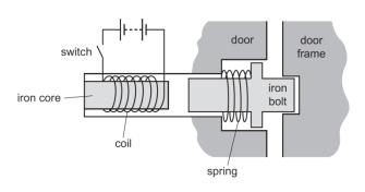
(a) The iron bolt moves to the left when the switch is closed. Explain why.
