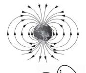
The North (seeking) pole of the Earth is actually a (magnetic) South pole. The South (seeking) pole of the Earth is actually a (magnetic) North pole. In NZ we live closest to a magnetic North pole.
