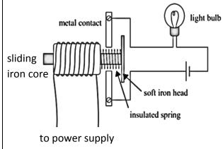
When the current flows, the **coil becomes magnetised** and **pulls soft iron core** to the left. The head of the core touches the two metal contacts thereby completing the light bulb circuit.
