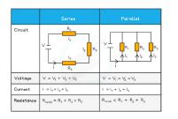
A complex circuit has elements of both series and parallel circuits. In any circuit, individual components still obey ohms law.
