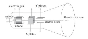
This diagram is a simplified diagram of the Y-plates in the cathode ray tube. These are two parallel metal plates.
