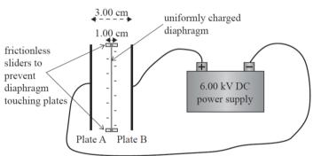
(d) At one point the stationary diaphragm has a uniform negative charge of -  $4.20 \times 10^{-5}$  C and is initially located in the middle of the slider. The mass of the diaphragm is  $5.80 \times 10^{-5}$  kg, and the width of the slider is 1.00 cm. The conducting plates are 3.00 cm apart. Find the maximum speed the diaphragm will have before it is stopped by the edge of the slider. State any assumptions you make.
