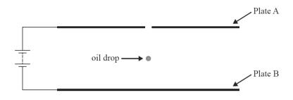
Millikan used x-rays to produce a negative charge on the oil drops.
