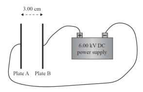
A simplified diagram of an electrostatic speaker is shown below. The plates are connected to a 6.00 kV high-voltage DC power supply.
