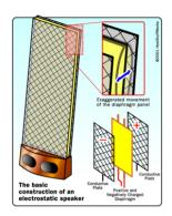
Sam has recently purchased an electrostatic speaker that produces sound by moving a diaphragm (thin sheet of polyester film) between two conducting plates that are 3.00 cm apart.
