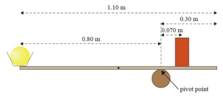
(b) Calculate the mass of the brick on the right side required for the beam to be level.
