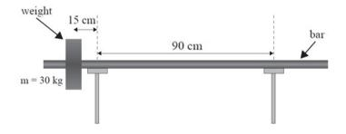
Use the concept of torque to calculate the weight of the bar. Assume it is a uniform bar.
