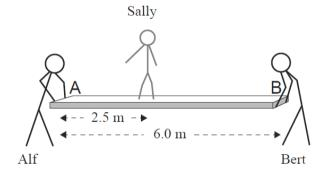
(a) In the diagram below, draw and name all forces acting on the plank.
