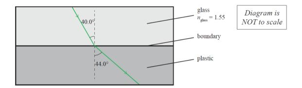
(b) If the angle of incidence in glass becomes greater than the critical angle, then the light is totally internally reflected, and no refraction takes place. Calculate the critical angle for the glass-plastic boundary to 3 significant figures.
