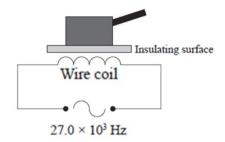
The coil used in a particular induction cooker is found to have an inductance of 1.30 mH.
