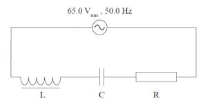
(b) The supply voltage in the circuit above leads the circuit current by  $35.0^{\circ}$ . The resistor has a resistance of  $1.50 \times 10^{2} \Omega$ . Calculate the total impedance of the circuit. A phasor diagram may be useful.
