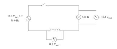
Casey adds in the  $9.45 \times 10^{-7}$  F capacitor to create an LCR series circuit. The light bulb barely glows. Casey switches the AC power supply to its maximum frequency setting of  $4.00 \times 10^{2}$  Hz.
