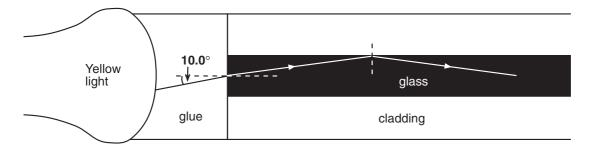
(e) Calculate the **angle of reflection** at the glass/cladding boundary.
