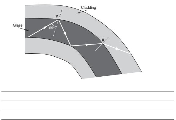
A decorative optical fibre light is made by gluing optical fibres to a yellow light. The refractive index of the glue is 1.36 and the refractive index of the core glass is 1.58. A ray is incident on the end of the fibre at  $10.0^{\circ}$ , as shown in the diagram below.
