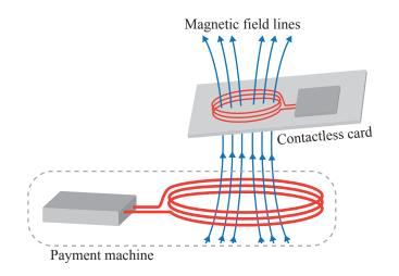
(c) The payment machine's induction coil has an alternating current of frequency  $13.6 \times 10^6$  Hz.
