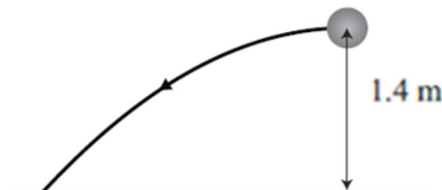
Calculate the velocity (magnitude and direction) of the ball just before it hits the floor.
