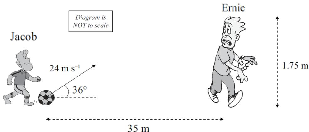
Will the ball hit Ernie or go over his head? In your calculations, you should start by showing that the horizontal component of the initial velocity of the ball is  $19.4 \text{ m s}^{-1}$ .
