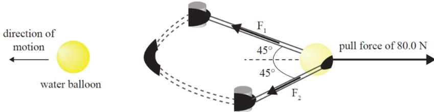
Draw a closed labelled **scale** vector diagram on the grid below. The 80.0 N horizontal force vector has been drawn for you.
