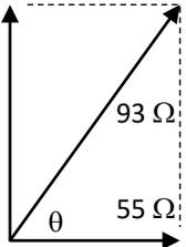
$\theta = \cos^{-1} \frac{55}{93} = 53.74$ Current lags the supply voltage by $54^\circ$ or 0.94 rad. | Recognition that voltage phase difference is the same as impedance phase difference.<br><br>OR<br>$\theta$ is labelled correctly in the diagram | Correct answer. $54^\circ$ or 0.89 rad                                                                                                            |                                                              |
