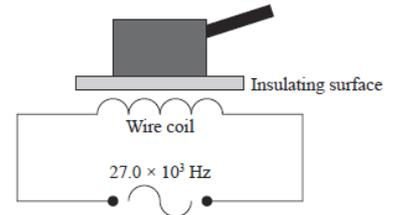
8. The capacitor in the induction cooker has a capacitance  $1.65 \times 10^{-8}$  F. Sam wanted to make a capacitor of this capacitance using two metal foil sheets. The two sheets of foil are separated by a layer of air  $1.00 \times 10^{-4}$  m thick. The permittivity of free space =  $8.84 \times 10^{-12}$  Fm<sup>-1</sup>. Calculate the area of the foil sheets that Sam should use.
