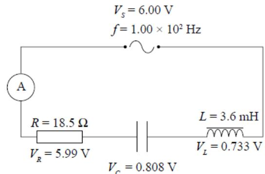
6. The inductor,  $L$ , in the circuit models the coil of wire under a road. The resistance of the rheostat is changed so that the current in the circuit drops steadily from its maximum value of 1.62 A to 0.13 A in 1.2 s. While the current is dropping, the voltmeter reads 4.0 mV. Calculate the inductance of the inductor.
